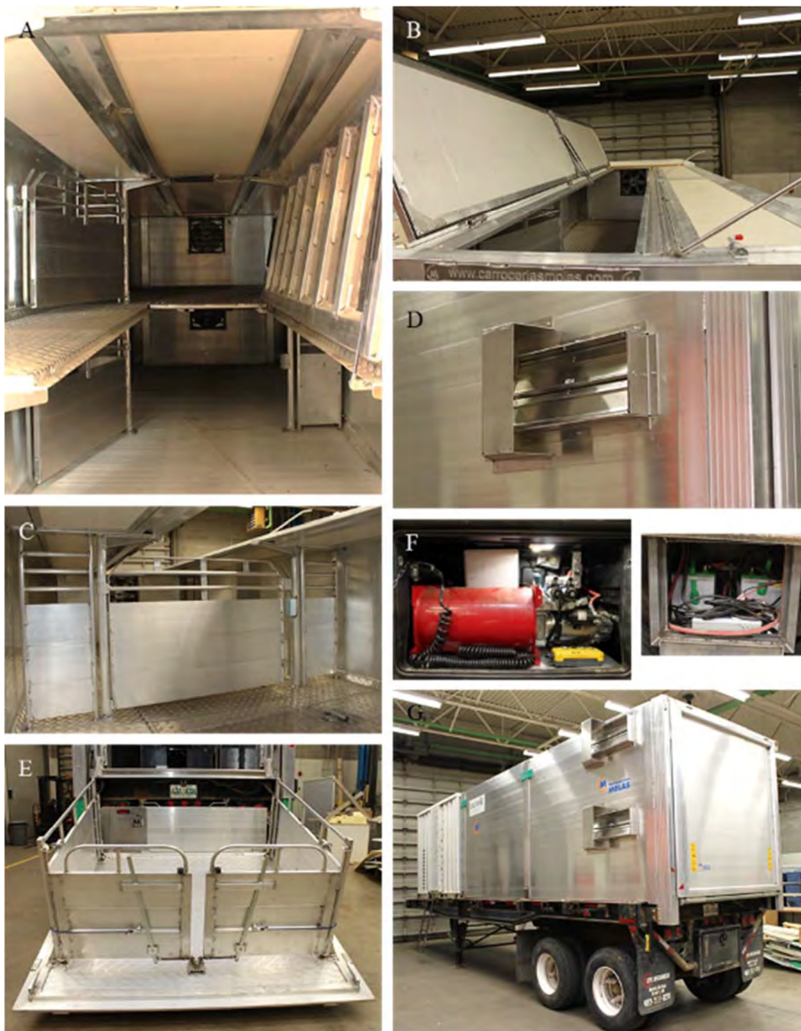
Figure 7.8. Photos of the animal compartment showing (A) its lower and upper decks, (B) hinged roof, (C) gate that partitions each deck into two compartments, (D) air exhaust damper, (E) hydraulic loading platform, (F) hydraulic system showing motor, pump, controller and power supply, and (G) exterior of the assembled compartment.
