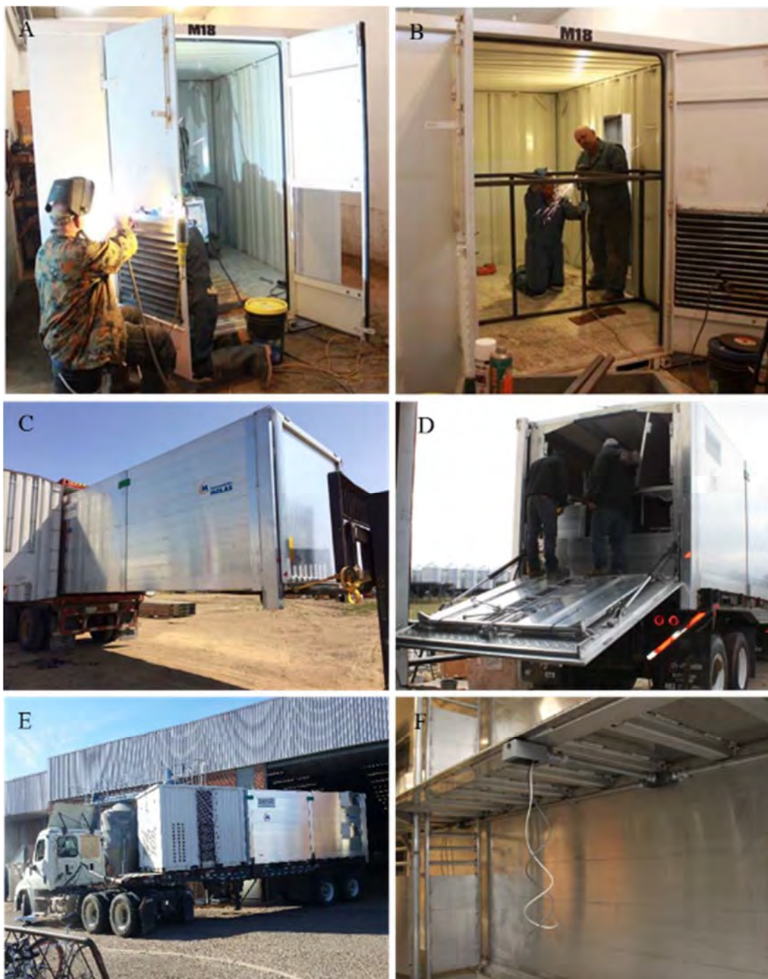
Figure 6.4. Photos during assembly of the prototype air-filtered trailer. Shown in (A) and (B) is the retrofitting of the metal storage container into the front compartment, (C) the animal compartment box being unloaded in Outlook, SK, (D) inspection of the trailer for placement of air outlet vents on the animal compartment, (E) moving of the assembled trailer to the College of Engineering to install sensors and (F) wiring of the sensors in the animal compartment.
